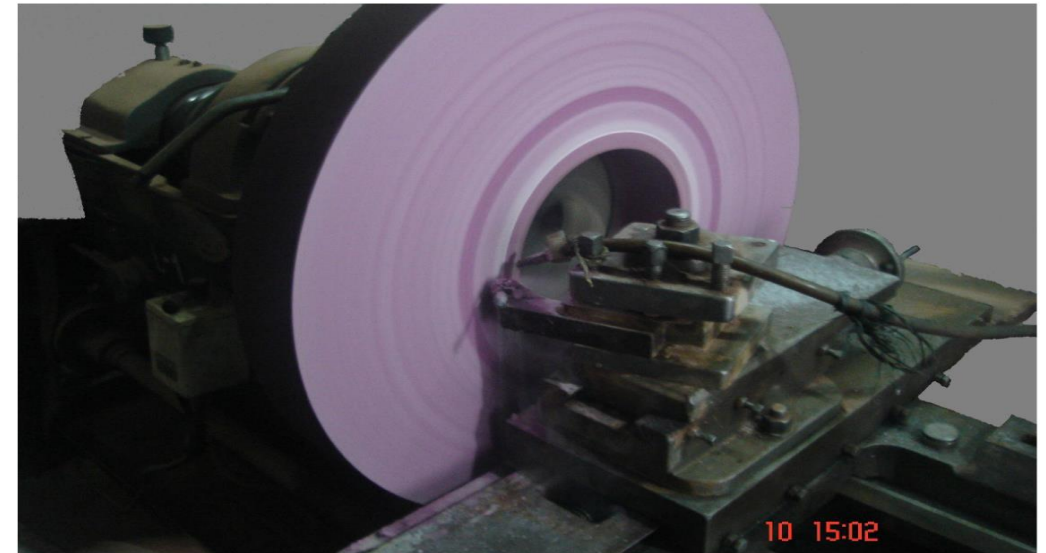
Setup for reforming spent crankshaft grinding wheels (2012)
