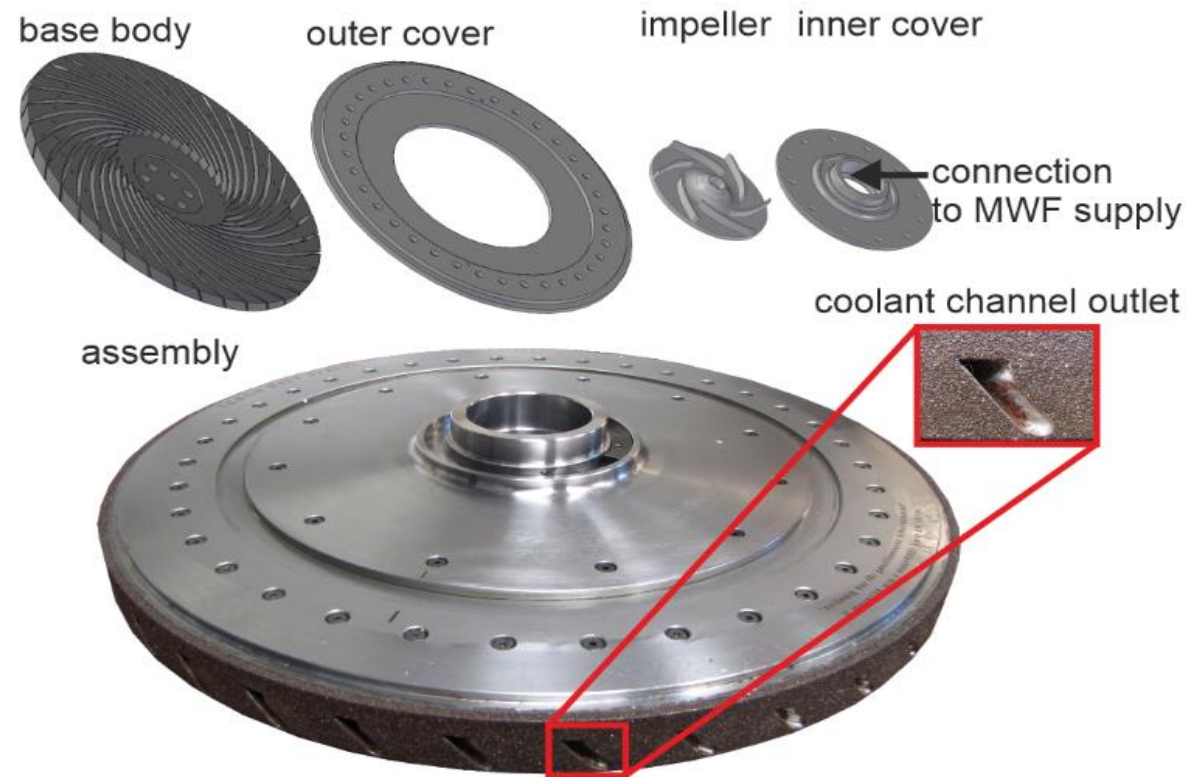
Parts and assembly of grinding wheel with internal coolant supply channels optimized for hydrodynamic properties (2011)
