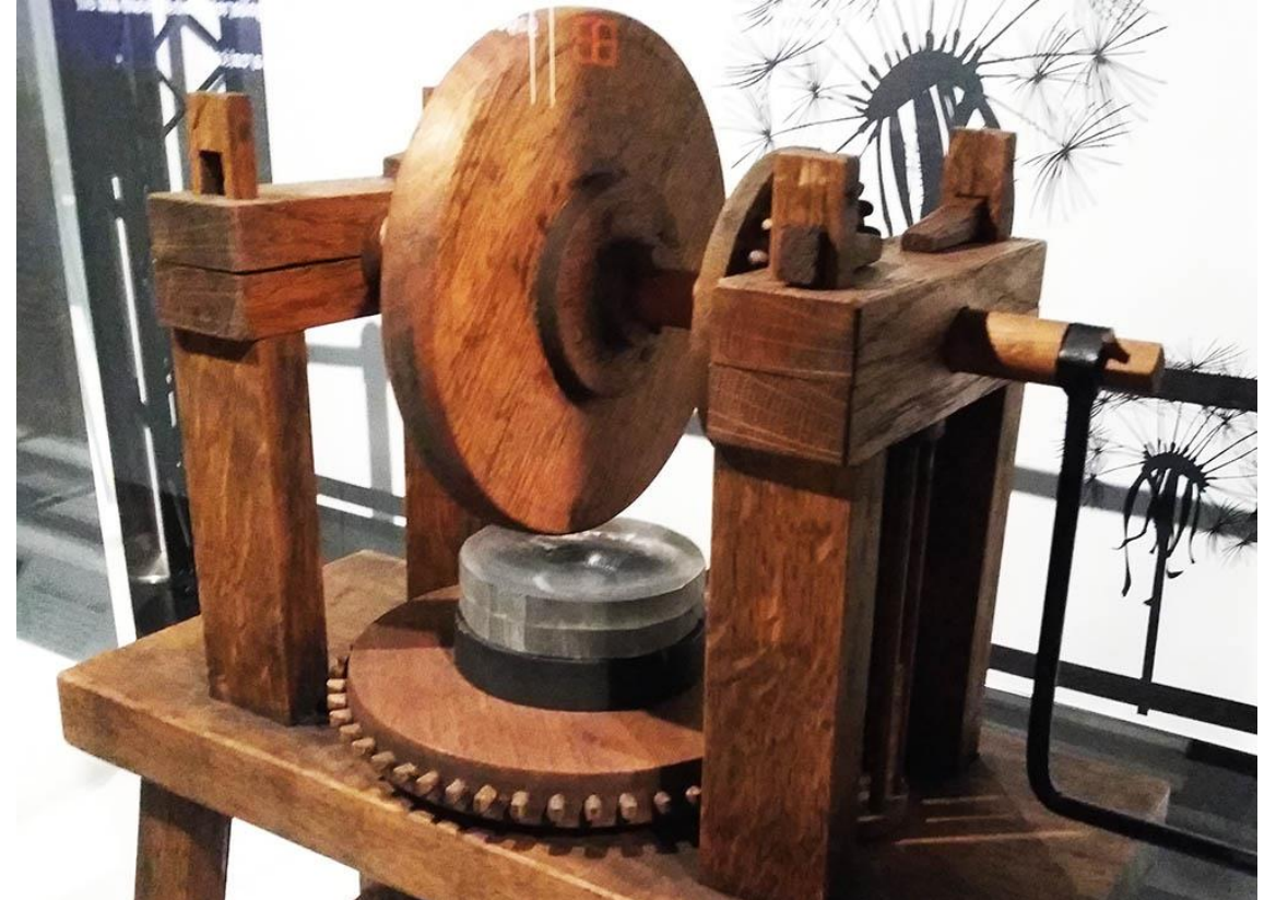
Optical Glass Grinding Machine (circa 15 th century)
