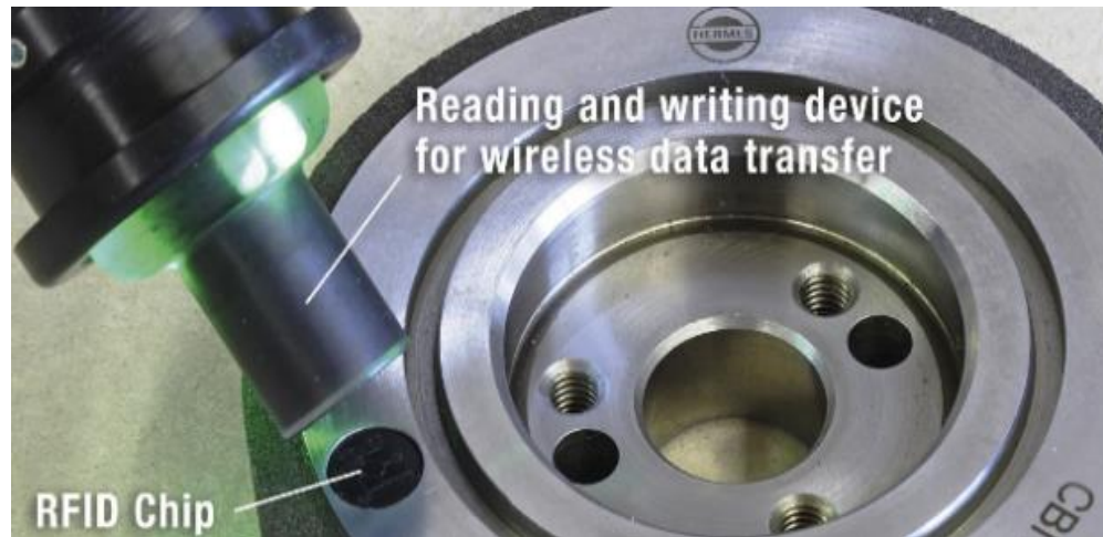
Possible measuring techniques within grinding wheels (2000)
